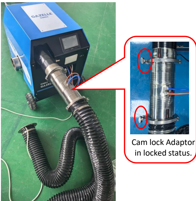
High flow Duct testing under positive pressure
