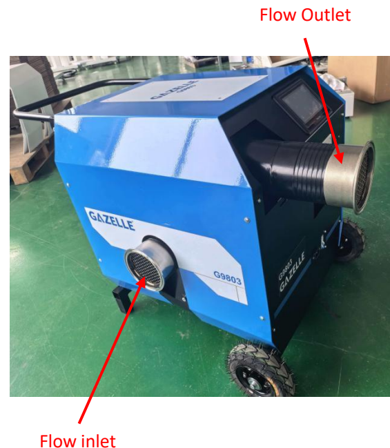
High flow Duct testing under Negative pressure
